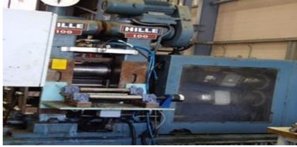
Figure 1. Hille 100 rolling mill
